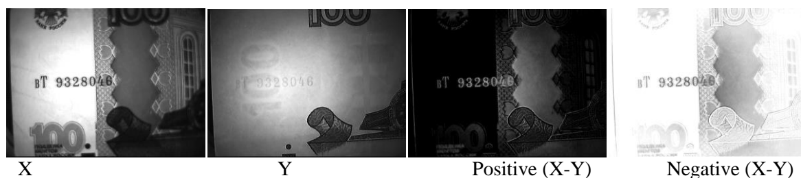
Figure 8. A fragment of a 100 Rub bill. X and Y - the original images obtained in non-overlapping ranges X(470 \pm 30\text{nm}) , Y(940 \pm 30\text{nm}) , and the corresponding differential images in positive and negative.
