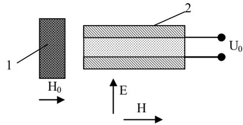
Fig.8. ME sensor of electromagnetic field, 1 — permanent bias magnet, 2 — ME sensor
