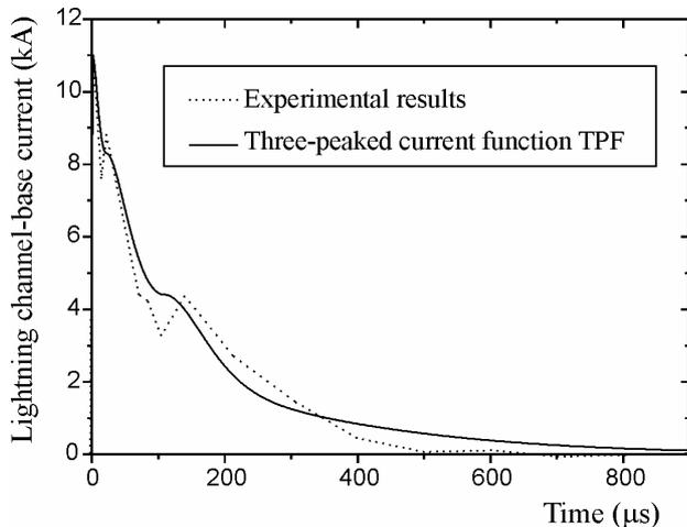
Fig.2. Lightning channel-base current TPF approximating the measured current [15]
