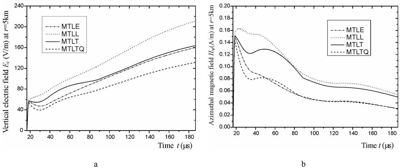
Fig.6. Vertical electric field (a) and azimuthal magnetic field (b) at  $r = 5$  km from the channel-base
