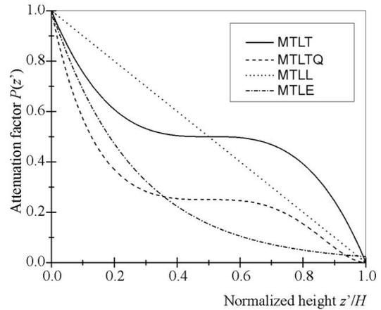
Fig.1. Attenuation factors in modified transmission line models
