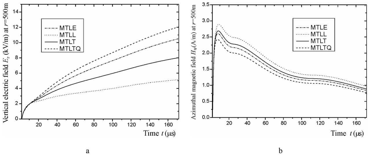
Fig.5. Vertical electric field (a) and azimuthal magnetic field (b) at  $r = 500$  m from the channel-base
