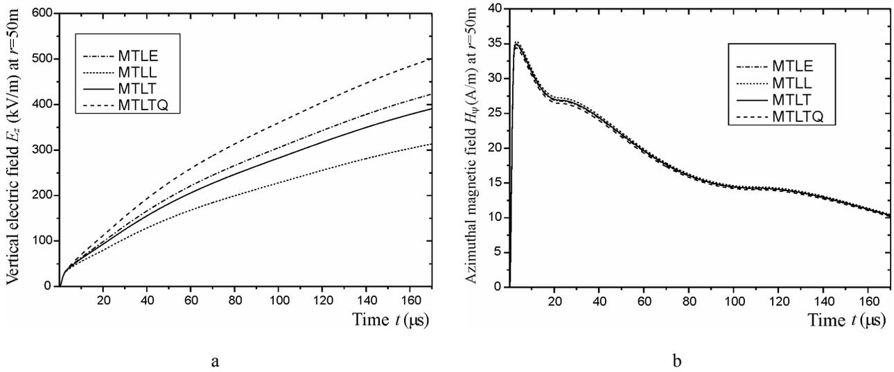
Fig.4. Vertical electric field (a) and azimuthal magnetic field (b) at  $r = 50$  m from the channel-base
