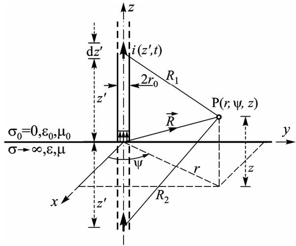
Fig.3. Lightning channel above perfectly conducting ground
