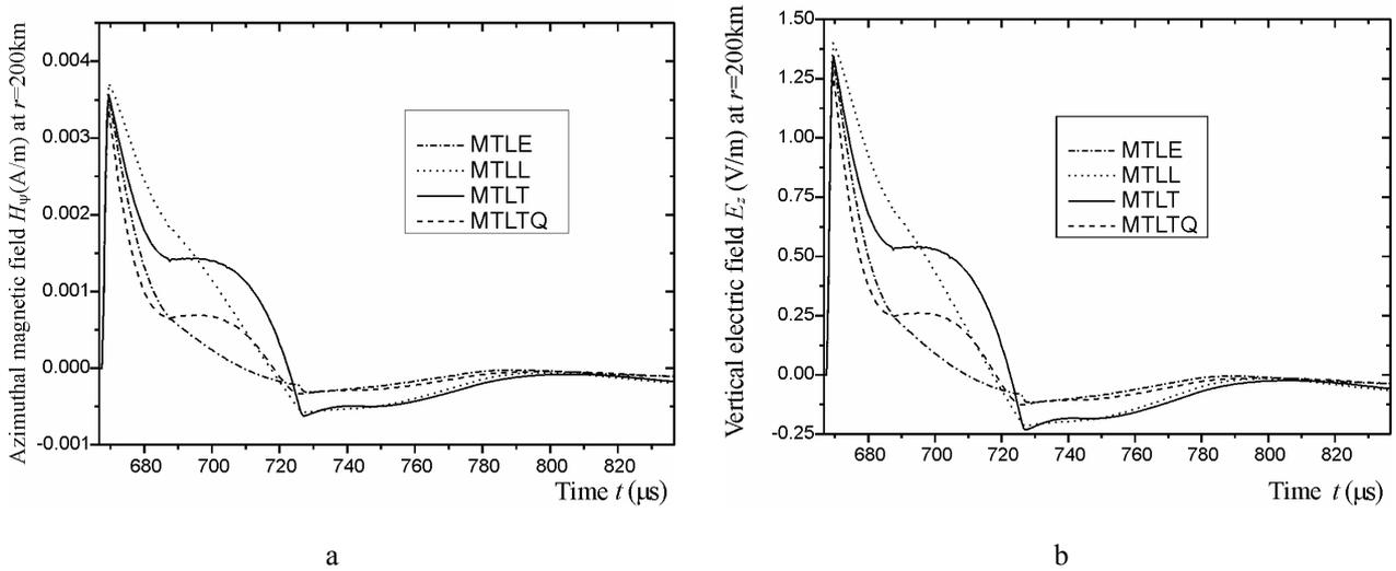
Fig.7. Vertical electric field (a) and azimuthal magnetic field (b) at  $r = 200$  km from the channel-base
